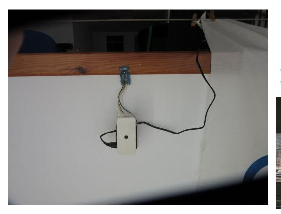
RPI3 (well I changed it to a RPIzero W) Controlled by a server ssh Use raspberry pi v2 camera Use BME280 I2C temp/pressure/humidity https://github.com/jfclere/pisolar/blob/main/b me280.py
